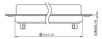
ΡN PIN А В С D 30.88 16.17 MHDB9SS 09 24.88 18.94 MHDB15SS 33.30 24.66 15 39.20 27.50 38.38 41.20 MHDB25SS 25 53.02 47.04 63.50 55.20 57.40 37 69.40 MHDB37SS
