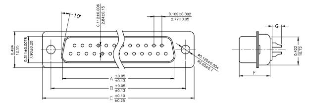
Material & Finish Shell: Steel Nickel or Tin plated
